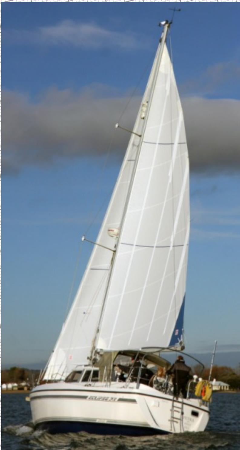
**CRUSADER SAILS'** fresh approach to the in-mast reefing mainsail combines a subtle blend of tried and tested high tech woven sailcloth, ultra lightweight carbon fibre sail battens and state of the art computer design to provide a smoothly rolling, high performance mainsail.
