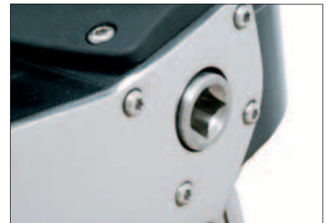
In case of power failure, Furlex Electric can be operated manually.
