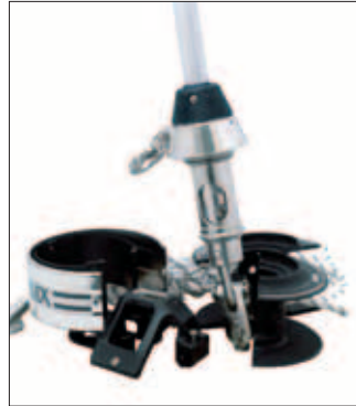
Remove line guard, line guide, rope and drum halves.
